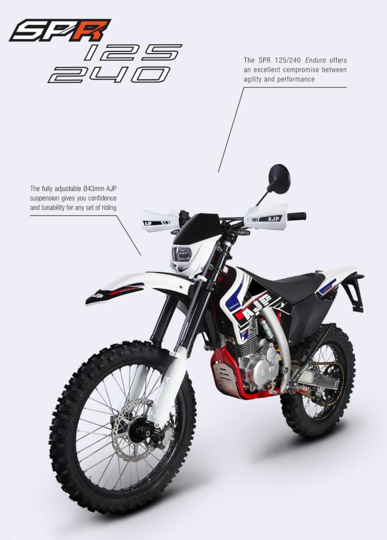
The 9,5L new ACERBIS under-seat fuel tank combined with the hybrid system of steel and aluminium frames allows any type of riding A complete new race-inspired chassis. This is AJP introducing enduro-leisure bikes to younger riders looking for new adventures BRAKTEC dual piston caliper with Ø260mm front disc,
