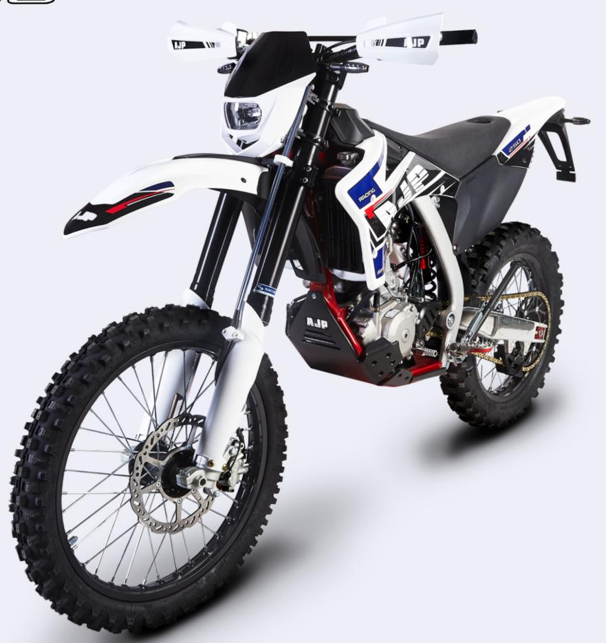
The SPR 250 raises the bar in the adventure stakes thanks to a ultra-lightweight chassis, a reliable 250cc monocylinder with electronic injection motor and a sophisticated suspension setup.
